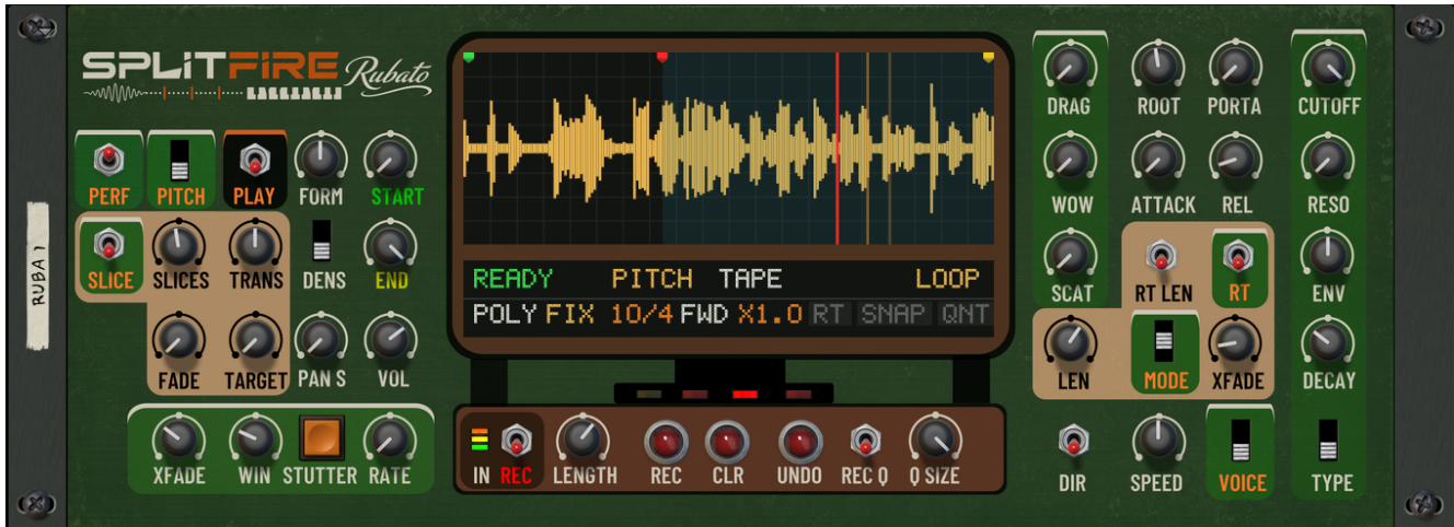
Rubato front panel — record / slice / play, with looper, stutter, character, envelope and filter sections.
